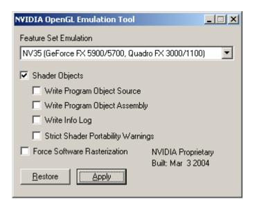
To enable the GLSL function, check the "Shader Objects" check box *and* press the "Apply" button. No changes to NVemulate settings take effect until the "Apply" button is pressed. Pressing the "Restore" button reverts the display settings to the driver's current applied state.
